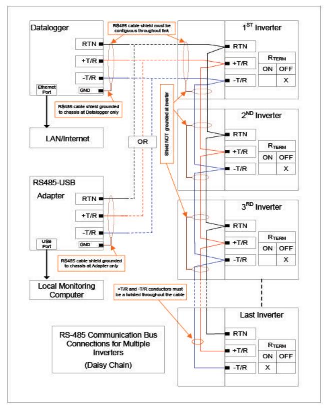
Figure 15C: Daisy Chain Communication wiring
