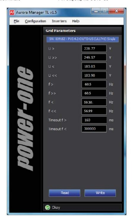
**Figure 4:06a:** Screen Capture of Aurora TL Manager with Changed Frequency and Timeout Values Once the frequency range and timeout values have been changed:
