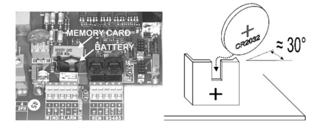
Figure 6:04 Lithium Battery Replacement
