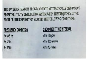
Figure 4.06b: Notification Label: Frequency Range and Timeout Parameter Change
