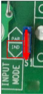
Figure 2:13a: Independent MPPT Configuration Switch
