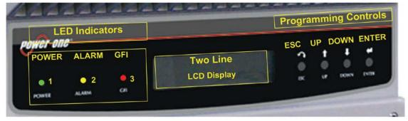
Figure 4:05: Location of the buttons and LEDs
