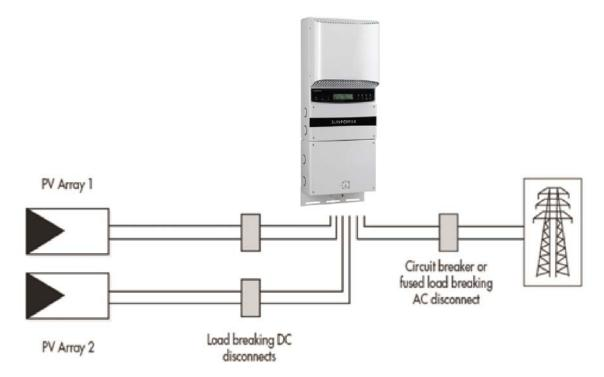
Figure 7:01 - Simplified Diagram of a Photovoltaic System
