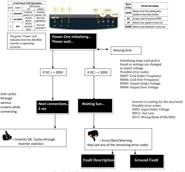
The yellow 'FAULT' LED indicates that the AURORA Inverter has detected a fault condition.
