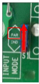
Figure 2:14a: Parallel MPPT Configuration Switch
