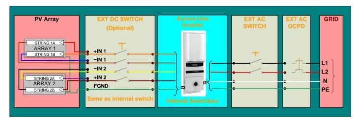
Figure 2:05: Electrical Connection Diagram PVI-3.0/3.6/4.2-OUTD-S-US
