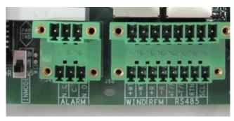
Figure 4:08: Alarm contact terminal block
