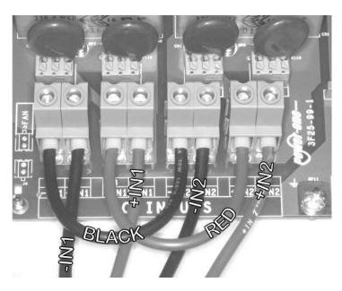
Figure 2:14b: Paralleling jumpers for  $\it PAR$  MPPT Configuration
