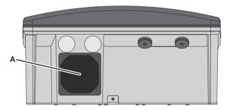
Figure 8: Position of the fan enclosure with fan
