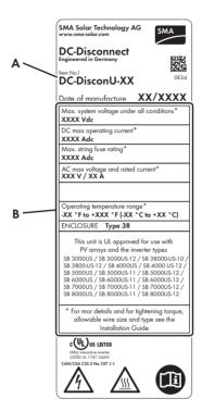
Figure 4: Layout of the DC Disconnect type label
